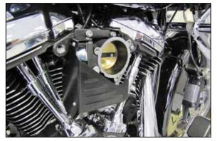
6. Install the K&N® servo cover and secure with the provided hardware to the original servo cover mounting bolt locations.
