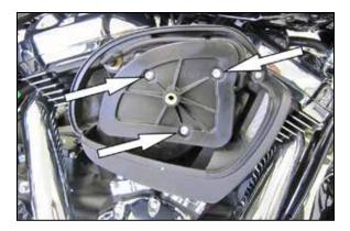
3. Remove the three bolts that secure the air filter element and then remove the air filter and crank case breather tubes.
