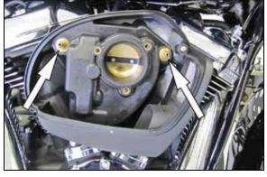
4. Remove the two breather bolts shown and then remove the rear air filter housing from the vehicle. NOTE: K&N Engineering, Inc., recommends that customers do not discard factory air intake.
