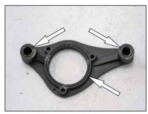
7. Install two of the breather O-rings and the throttle body O-ring into the base plate as shown. NOTE: Use a few small dabs of grease to secure the O-rings in place while installing the base plate to the engine.
